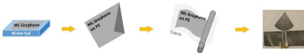
Figure 2. The fabrication process of graphene-based soft antennas. From left to right: (i) ML graphene grown on Ni foil; (ii) ML transferred on PE sheets; (iii) graphene lamination on textiles, (iv) antenna patterning
