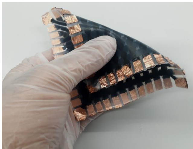
Figure 1: SCEEP, a silicon-based capacitive skin, is highly stretchable and foldable.
