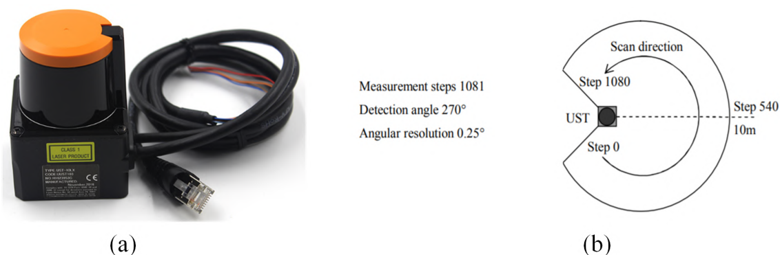
Figure 5.6: (a) UST-10LX LiDAR, (b) Laser scanning image
