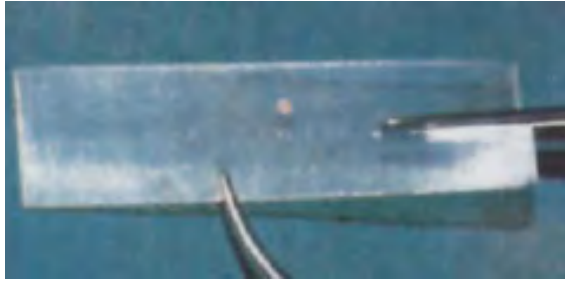
Figure 3.2 showing a) one of the 0.5mm thick self-reinforced PLLA plates used b) to repair the bony defects in the skull of a patient suffering from trigonocephaly treated by cranioplasty (From Waris et al. , 1994).
