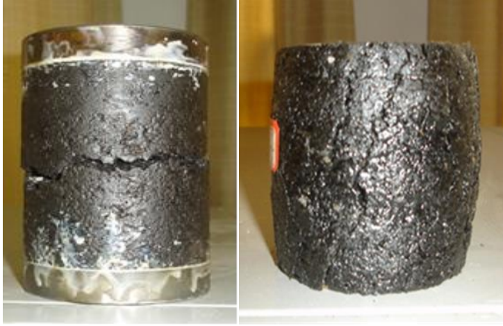
Fig.11 Tensile failure. Fig.12 Shear failure.
