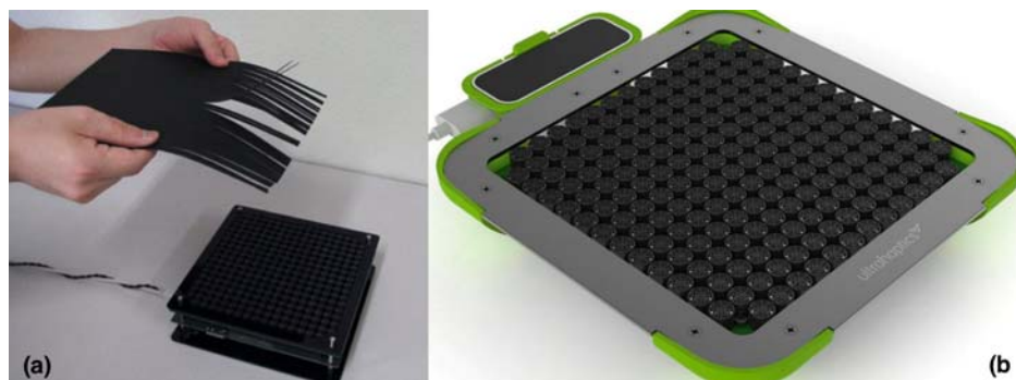
Fig. 4.8. The focused ultrasounds can flip up thin paper strips (a) (Hoshi and Shinoda 2016) and the commercially available Ultrahaptic display (b)(Ultrahaptics, UK).
