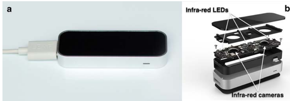
Fig. 8.34. Picture of the Leap Motion hand tracking system (a) and exploded view of the system (b).
