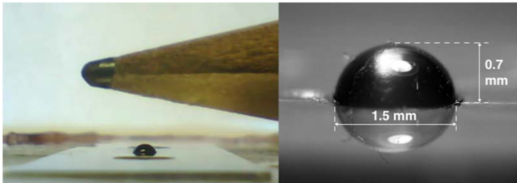
Fig. 11.1. Pictures of the prototype Braille dot at rest (with no voltage applied).
