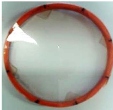
Fig. 8.6. The elastomer is transferred onto a plastic ring used to keep the film pre-stretched during the fabrication process.
