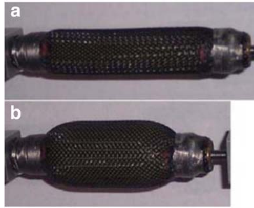
Fig. 6.4. Pictures of the McKibben artificial muscle in the rest state (a) and when pressurization produces the contraction (b) (Kang et al. 2009).
