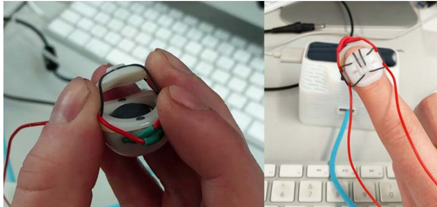
Fig. 12.2. Pictures of the new casing for the tactile display.
