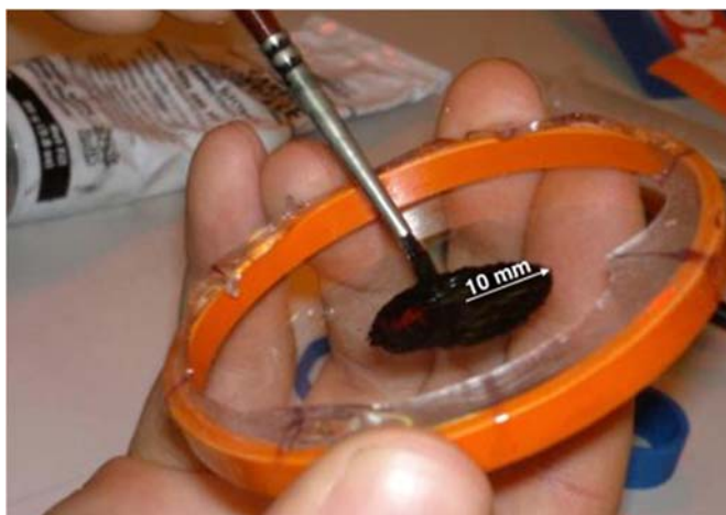
Fig. 8.7. The carbon grease electrode is smeared onto the elastomer surface using a brush.
