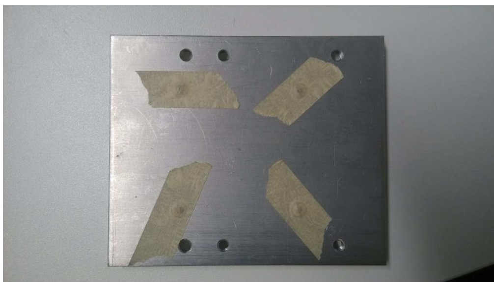
Figure 5-8 Photograph of the rectangular metal target used in the raster scanning experiment.
