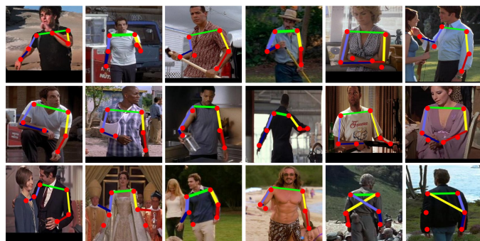
Fig. 6. Visualization of pose results in images from the FLIC. Each pose is represented as a stick figure, inferred from predicted joints. Different limbs in the same image are colored differently, and the same limb across different images has the same color. The red nodes represent the location of joints(ground truth). The first two rows are accurate results and the last row presents some false detections. This figure is best viewed in color.
