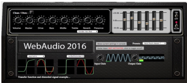
Figure 4: A guitar tube amplifier simulation made with WebAudio. The WASABI database embeds tools for re-creating/studying the sound of the instruments played in classic rock songs.
