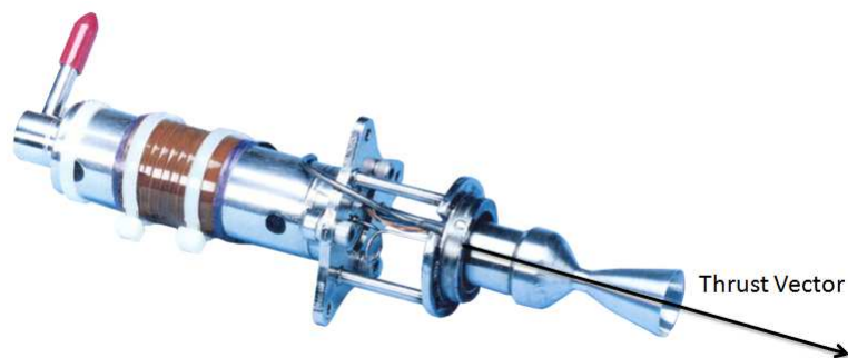
Figure 3.11.: 5N Hydrazine thruster showing the definition of thrust vector/thruster centreline used.
