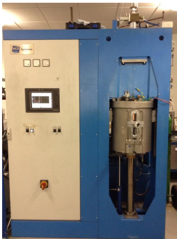
Fig. 3.2.1 Spark Plasma Sintering furnace (HPD 25/1 FCT, Germany).
