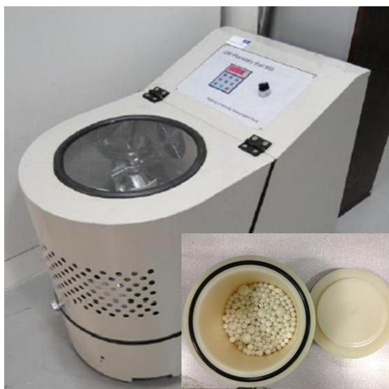
Fig. 3.1.1 Planetary ball milling machine (QM-3SP4, Nanjing University Instrument Plant, China). Inset shows the nylon ball-milling pot with ZrO_2 milling balls.
