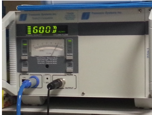
Figure 2.9 The processing unit for the transit time flow probe
