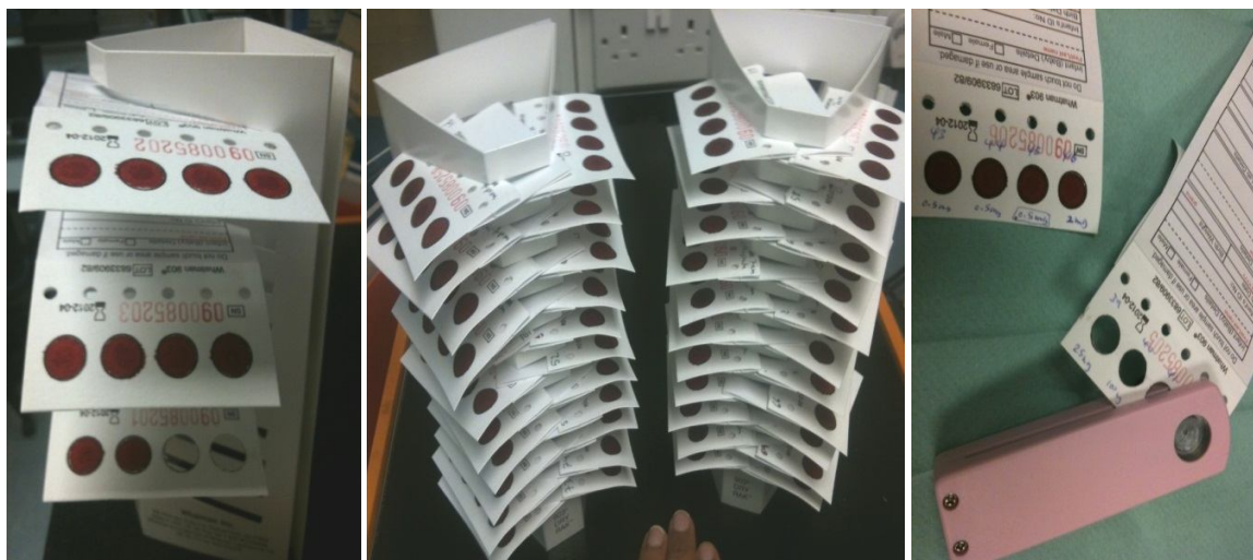
Figure 29: 50µl aliquots of spiked blood spotted on Guthrie cards, dried, and punched out
