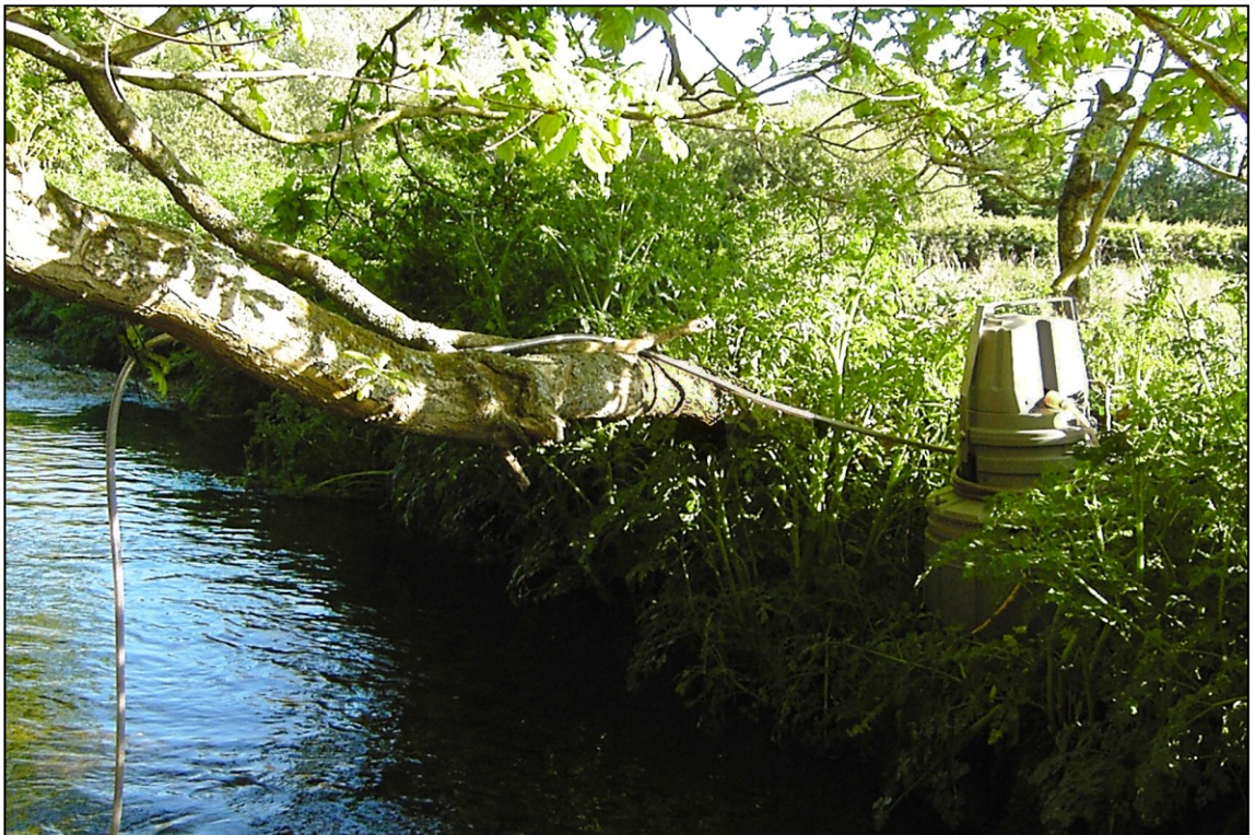
Figure 3. 9 – The Xian waste water sampler in position on the Bere Stream in July 2010. Photograph by G. Davies
