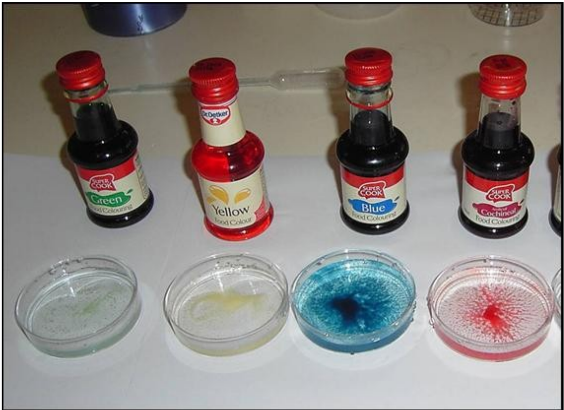
Figure 3.4 – Corn pollen particles that have been dyed in a range of conspicuous colours using commercially available food dyes. Corn pollen particles within these samples appear aggregated due to shaking and stirring. Photograph taken by G. Davies.
