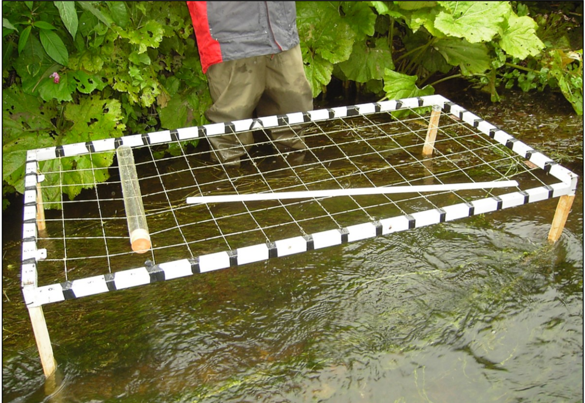
Figure 3.5 – The mounted quadrat used for detailed stand investigations on the Bere Stream and the River Frome. The quadrat is in place on the River Frome in this picture with the study patch beneath during the July 2009 survey. Photograph taken by G. Davies.
