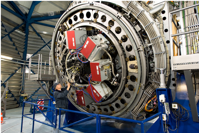
Fig. 3. Back-end of VISTA, with the VIRCAM at Cassegrain focus. The rear of the cryostat is seen (black), with the filter wheel bulge at the far side. The five red electronics boxes are mounted on the cryostat. The camera coolers and cryo-pumps are mostly hidden behind the electronics boxes. The large annular structure surrounding the camera is the Cassegrain cable-wrap; fixed sections of Helium hoses are seen curving around the back of the M1 Cell, and enter the cable-wrap at the connector box at lower right.
