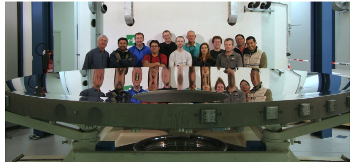
Fig. 4. VISTA primary mirror on its wash-stand, after the first coating in April 2008. The telescope pier is behind the group. The apparent “kink” near the front arises from two reflections off the mirror.
