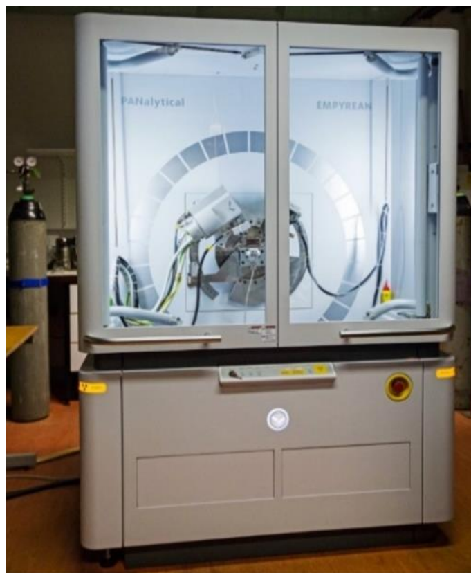
Fig. 2.3 The PANalytical Empyrean Ag-anode X-ray diffractometer, located at Queen Mary University of London. The X-ray wavelength is \lambda = 0.5609 \text{ \AA} , the maximum diffraction angle 2\theta = 156^\circ , which corresponds to Q_{\max} = 21.9 \text{ \AA}^{-1} .
