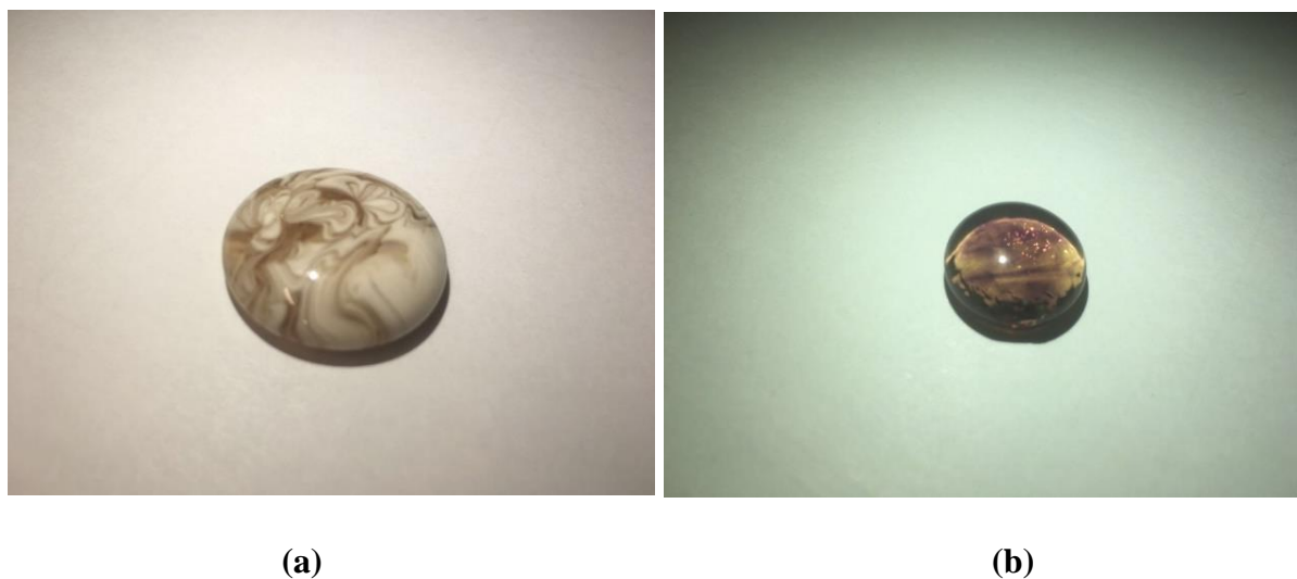
Fig. 4.1 Crystallised samples (a) x = 30 and (b) x = 25 in the system (60-x) \text{Li}_2\text{O} : x\text{MnO} : 40\text{P}_2\text{O}_5
