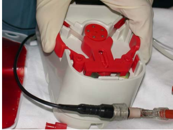
Figure 2.13 Lithium ion sensitive electrode (bottom right) and battery operated peristaltic pump.
