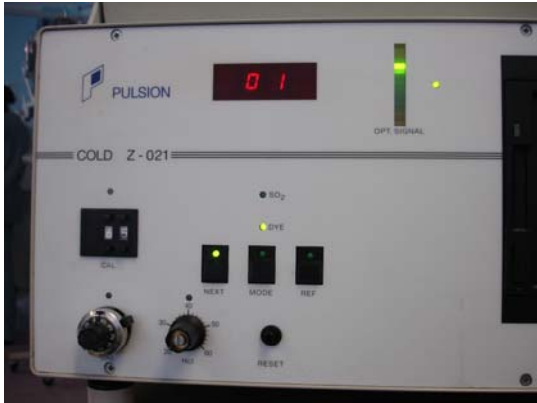
Figure 2.5 Strong pulsatile signal indicated by green ‘opt signal’ and good baseline calibration (red 0.01).
