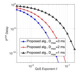
Fig. 8. Delay-outage probability versus QoS exponent  $\theta$  for various values of  $D_{\max}$  for our proposed algorithm.
