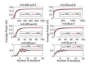
Fig. 6. Convergence behaviour of the proposed algorithm for the special case of two RRHs under different step parameters. Left three subplots correspond to the QoS exponent  $\theta = 0.005$ , and the right three correspond to  $\theta = 0.05$ .
