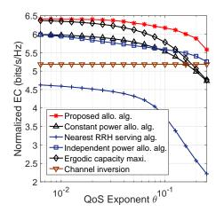
Fig. 11. Normalized EC for various algorithms vs QoS exponent  $\theta$  for the more general case of I = 5.
