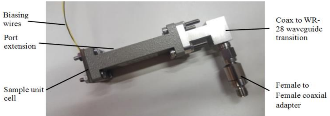
Fig. 3-11: Experimental setup for the waveguide-based characterisation of the silicon.
