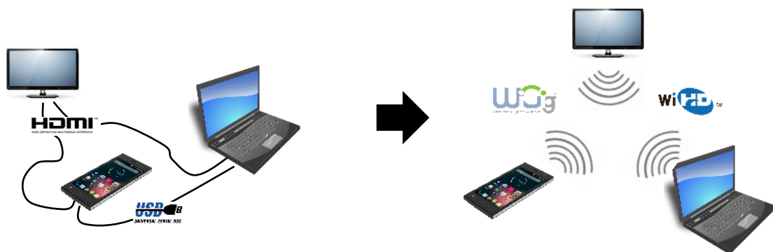
Fig. 1-1: Block diagram for a typical evolution to a WirelessHD system.
