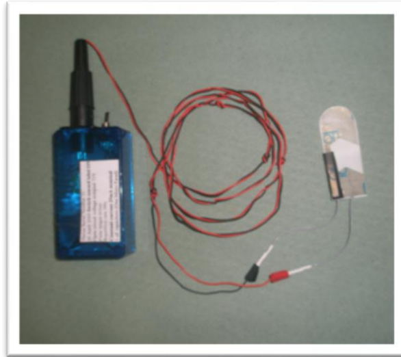
Figure 11: A Custom Built Electrical Stimulator Device. The custom built device (THRIVE) developed by Dr Arthur Tucker and Dr Duncan Bain consists of two geometrically corrected electrodes connected by wires to a stimulator box.
