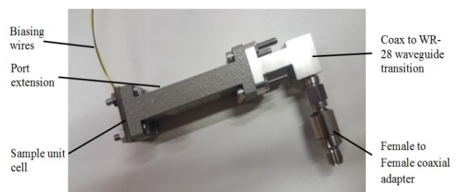
Fig. 3 Experimental setup for the unit-cell characterisation
