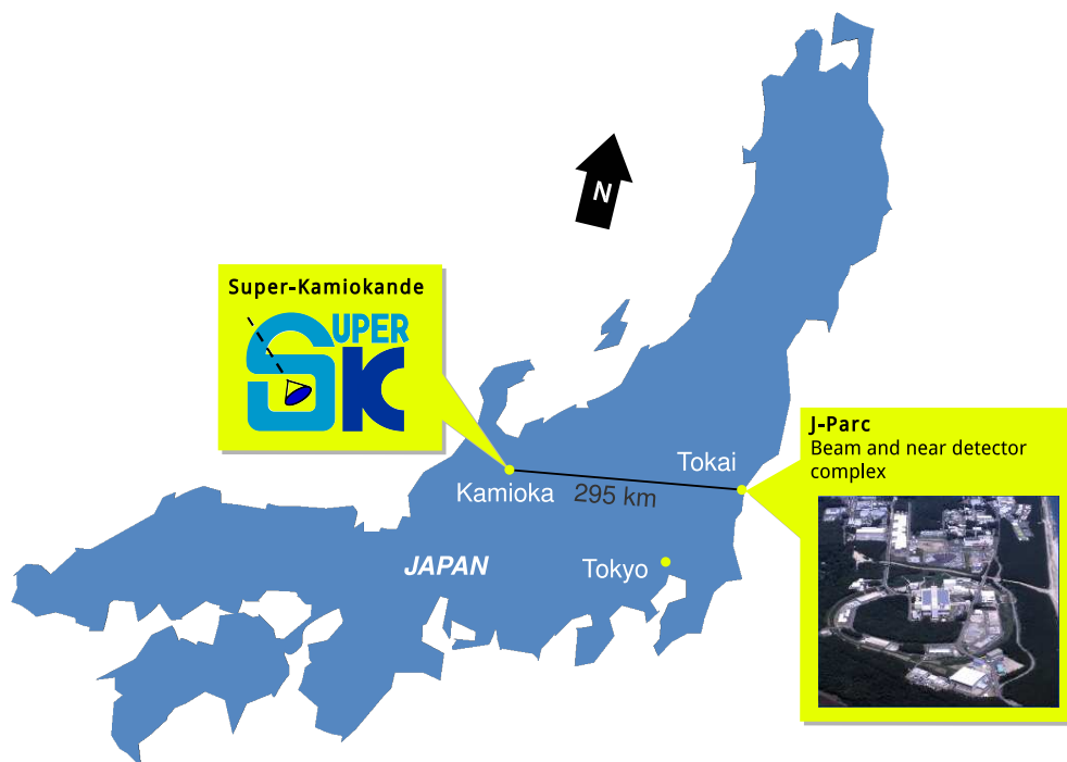
Figure 3.2: Map of Japan showing the location of the two sites used in the T2K experiment. A baseline of 295 km separates them.
