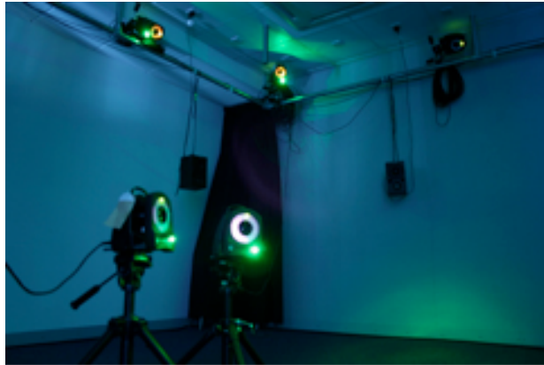
Figure 1. Infrared cameras in the Augmented Human Interaction (AHI) laboratory
