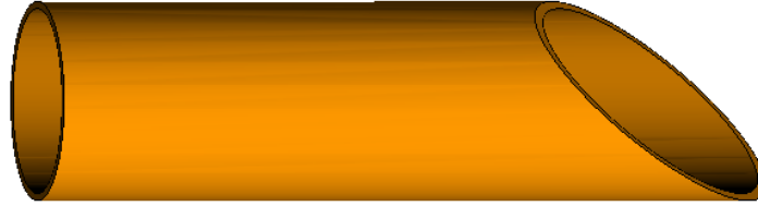
Figure 2-11: The profile of a bevel-cut Vlasov launcher.
