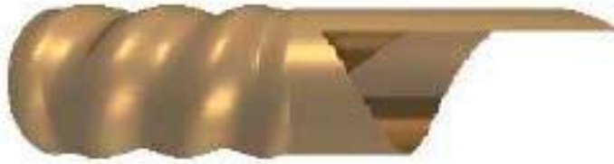
Figure 2-16: The profile of a Denisov launcher [103].
