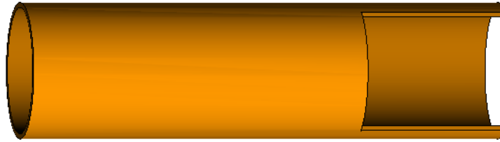
Figure 2-9: The profile of a step-cut Vlasov launcher.
