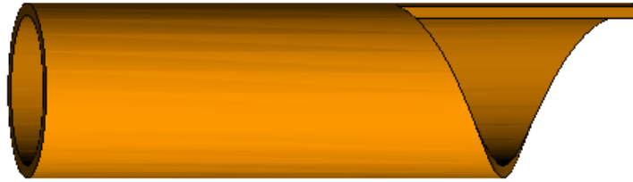
Figure 2-13: The profile of a helical-cut Vlasov launcher.
