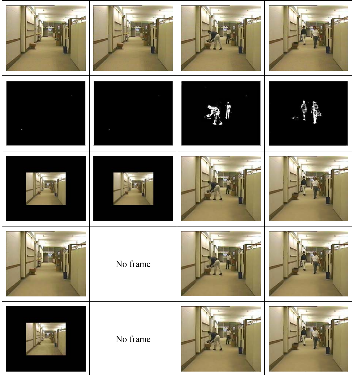
Figure 37: Frames of the reconstructed “Hall” sequence obtained. First row: the original frames. Second row: binary mask. Third row: Spatial adaptation. Fourth row: Temporal adaptation. Fifth row: Combined adaptation.
