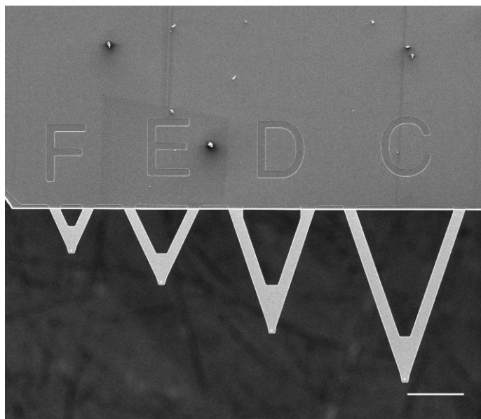
Appendix Figure 1. SEM image of AFM cantilevers used. Scale bar, 100 \mu\text{m}
