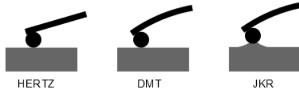
Figure 2.11. Illustration of the initial contact of Hertz, DMT, and JKR theories.
