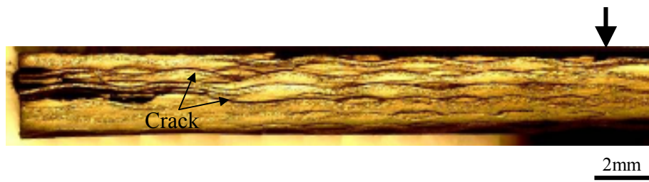
Figure 5.28 Cross-section image of 12J impacted specimen for PE/C (70:30) hybrid veil interleaved vinyl ester system (Broad arrow indicates impact point)
