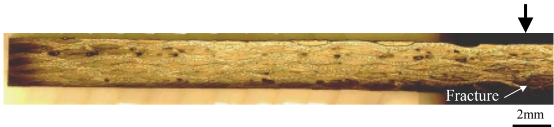
Figure 5.38 Cross-section image of 12J impacted specimen for PA veil interleaved epoxy2 system (Broad arrow indicates impact point)
