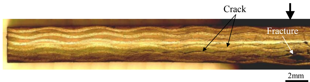
Figure 5.30 Cross-section image of 12J impacted specimen for PE/C (80:20) hybrid veil interleaved epoxy system (Broad arrow indicates impact point)
