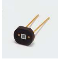
Figure 35: Hamamatsu multi-pixel photon counter. The grey central square is the 1.3\text{mm}^2 667 pixels and the MPPC is read out through the two pins.
