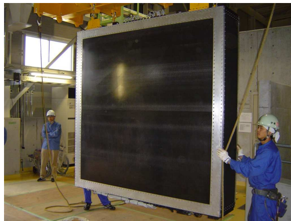
Figure 30: The completed DSECal being put onto the crane at J-PARC, ready to be installed in the pit.
