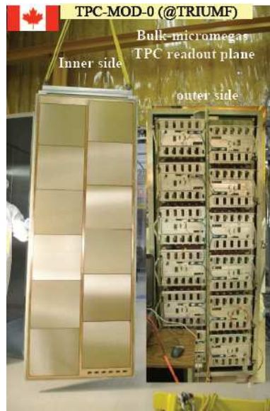
Figure 21: The TPC showing the large scale implementation of bulk micromegas.
