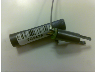
Figure 36: A fully assembled MPPC. The outer protective shroud bearing the unique manufacturer’s number and bar-code of the MPPC can be seen on the left. The two pins of the MPPC protruding from the smaller shroud can be seen in the centre of the frame connected to the PCB. The coaxial cable connecting the MPPC to the electronics readout boards is connected to the PCB.
