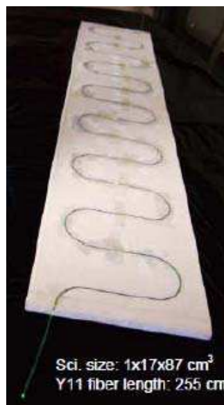
Figure 22: An SMRD plane showing the WLS readout.
