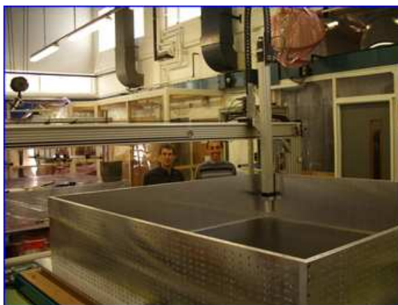
Figure 26: The 2D scanner in action testing one of the layers of the DSECal, sitting inside the bulkhead.
