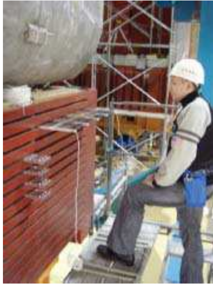
Figure 23: The SMRD being fitted within the gaps of the UA1 magnet.
