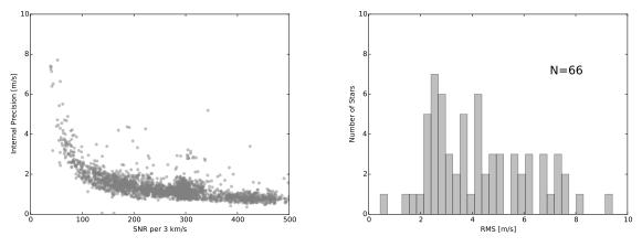
Figure 13. Radial velocity precision as a function of SNR (left) and velocity rms (right) for the Lick Planet Search team with the Levy Spectrograph at the Automated Planet Finder. (Courtesy of Greg Laughlin)
