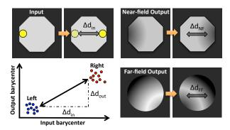
Figure 17. Cartoon illustrating measurement of scrambling gain by translating the test fiber across a fixed illumination spot and recording the output at each position. Measurements are made for the fiber near field and far field. (Courtesy of Sam Halverson)
