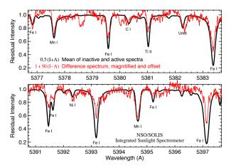
Figure 19. Full disk solar spectrum and the magnified difference between active and inactive states. Individual lines respond differently to activity changes, providing a way to help distinguish surface phenomena from Keplerian velocity shifts (Courtesy of Jeff Valenti).
