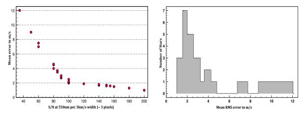
Figure 10. Precision and radial velocity scatter for PARAS. (Courtesy of Abhijit Chakraborty) The plot on the left shows the nightly RV scatter as a function of SNR in 3 km s<sup>-1</sup> bins and the plot on the right is a histogram of the long term rms scatter for 27 bright stars.
