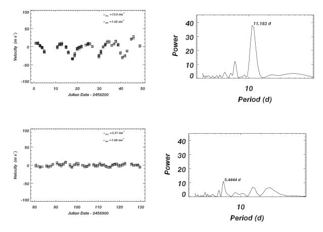
Figure 18. Radial velocity measurements of Epsilon Eridani using the CHIRON spectrometer at CTIO have internal errors of 1 m s<sup>-1</sup>. In 2012 (top panel) a clear 11.4-day periodicity is seen, which matches the rotation of the star. The rms variability is 13.6 m s<sup>-1</sup>. This signal attenuates over time and in 2014 (bottom panel) was not detectable. (Courtesy of Debra Fischer)
