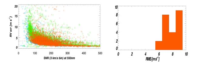
Figure 1. Single measurement precision as a function of SNR (left) for dewar 13 (blue triangles) used from 1994 - 1997, dewar 6 (green diamonds) from 1998 - 2000, and dewar 8 (red circles) from 2001 - 2011. The radial velocity rms scatter (right) is plotted for data from the Hamilton spectrograph at Lick Observatory; most stars have rms scatter greater than the 10 m s<sup>-1</sup> cutoff (Figures provided by Debra Fischer).
