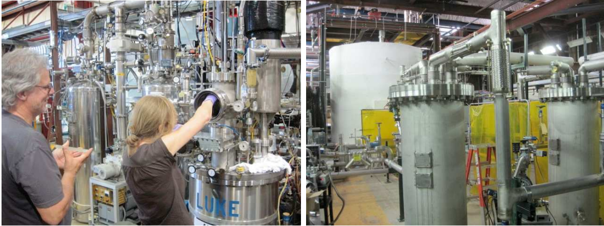
FIGURE 2. (color online). (Left) The Fermilab MTS cryostat, “LUKE”. In this picture, a scientist prepares a test sample in the sample cage. (Right) The Liquid Argon Purity Demonstrator (LAPD). 2 Zeolite filters are seen in front and the 30 ton vessel is seen in back.
