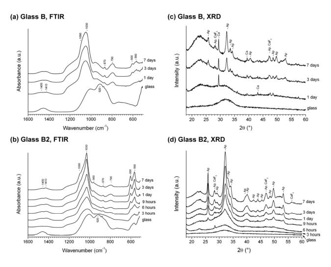
**Figure 2**: FTIR spectra (a, b) and XRD patterns (c, d) of glasses B (top, low phosphate) and B2 (bottom, high phosphate) before ("glass") and after immersion in tris buffer at different time points.
