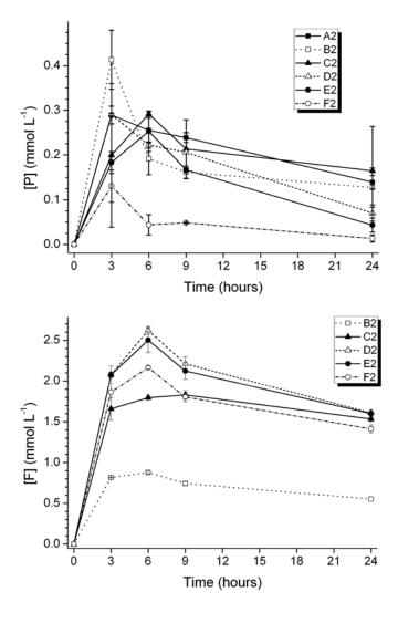
**Figure 6**: Elemental concentrations ± standard deviation of P and F in tris buffer *vs.* incubation time up to 24 hours of high phosphate content glass powders. (Lines are drawn as a guide to the eye.)
