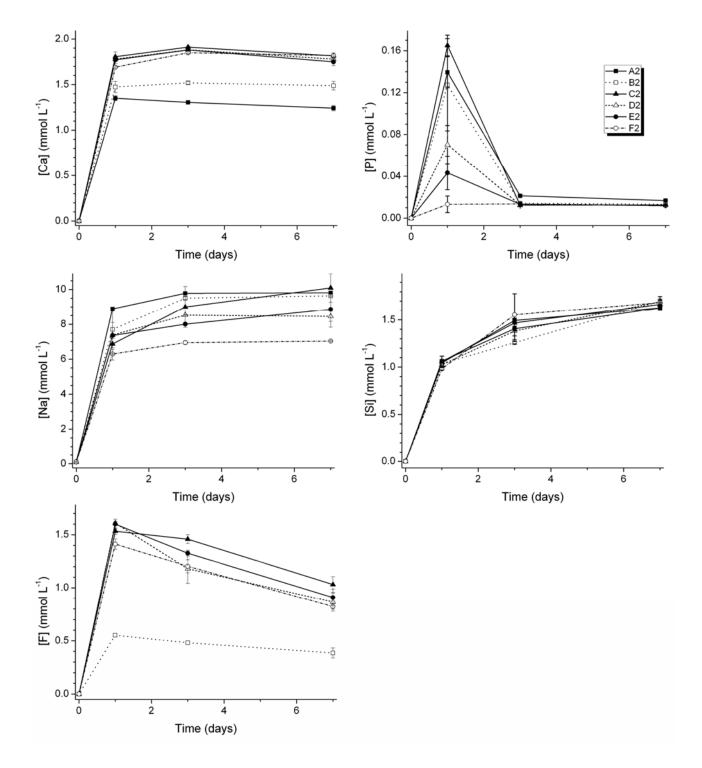
**Figure 5**: Elemental concentrations ± standard deviation of Ca, P, Na, Si and F in tris buffer *vs*. incubation time of high phosphate content glass powders. (Lines are drawn as a guide to the eye.)
