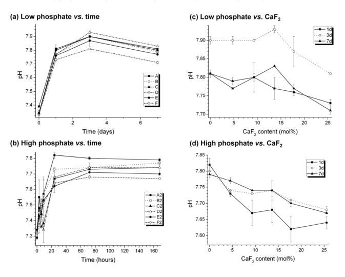
Figure 1: pH of tris buffer solution after immersion of (a) low phosphate and (b) high phosphate glasses vs. time and (c) low and (d) high phosphate content glass powder vs. CaF<sub>2</sub> content in the glass. (Lines are drawn as a guide to the eye.)
