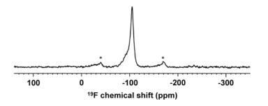
Figure 4. <sup>19</sup>F MAS-NMR spectrum of glass B2 at 1 week immersion in tris buffer. Spinning side bands are marked by an asterisk.
