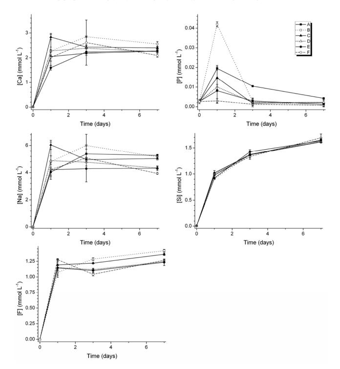
**Figure S4**: Elemental concentrations ± standard deviation of Ca, P, Na, Si and F in tris buffer *vs*. incubation time of low phosphate content glass powders. (Lines are drawn as a guide to the eye.)
