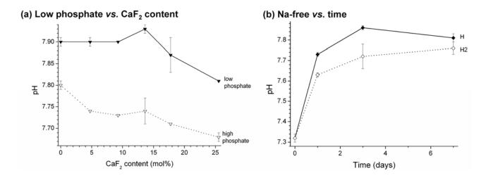
Figure S2: pH of tris buffer solution after immersion of (a) low and high phosphate content glasses for 3 days vs. CaF<sub>2</sub> content in the glass and (b) glasses H (low phosphate content) and H2 (high phosphate content) vs. time. (Lines are drawn as a guide to the eye.)
